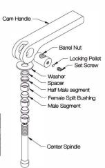
Moving the cam handle expands pin diameter up to .006 inches, to take up slack and secure the pin in place. If additional adjustment is required, remove set screw and turn the cam handle.
