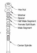
Tightening the hex nut with a wrench expands pin diameter up to .006 inches, to take up slack and secure the pin in place. Hold center spindle stationary with a hex key while tightening.
